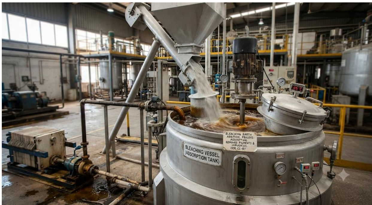
Image showing bleaching earth being added to crude oil Caption: Plate 5.2 Bleaching process in oil refining
