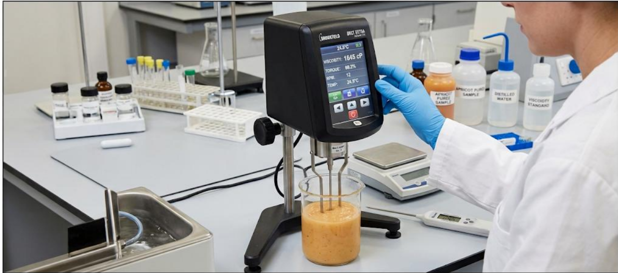
Plate 1.1: Laboratory viscometer for measuring viscosity
