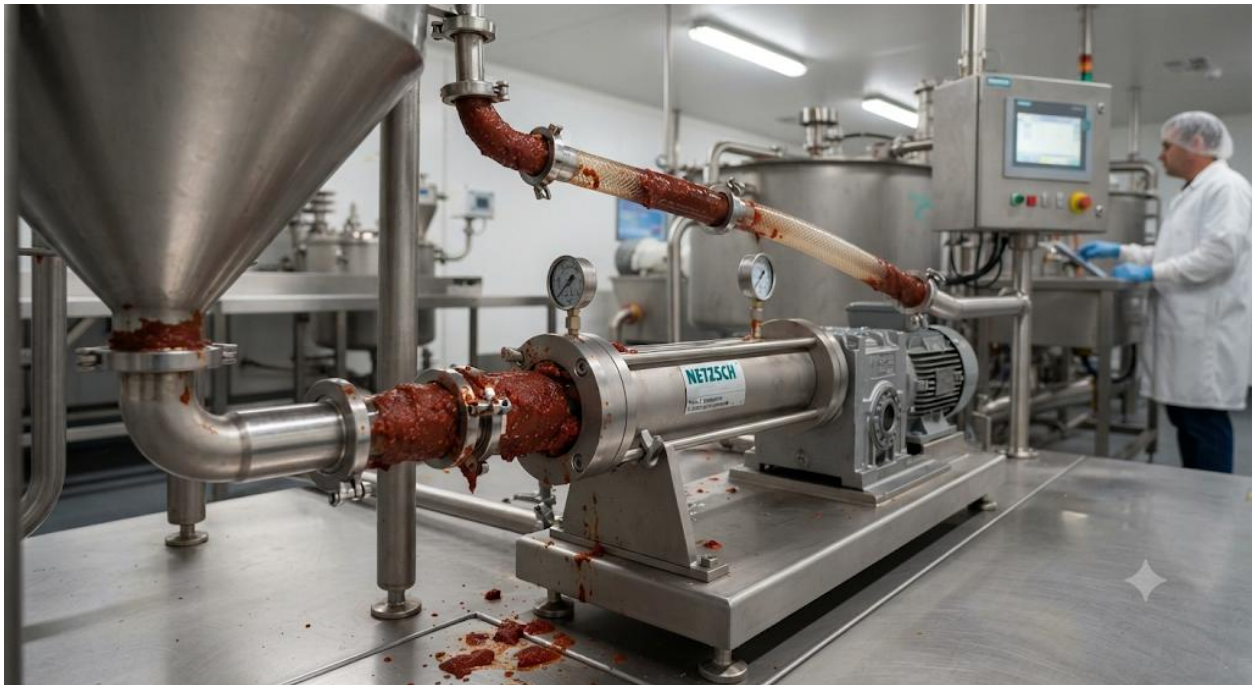
Image of industrial screw pump used in sauce processing Plate 4.3: Screw pump in tomato paste processing
