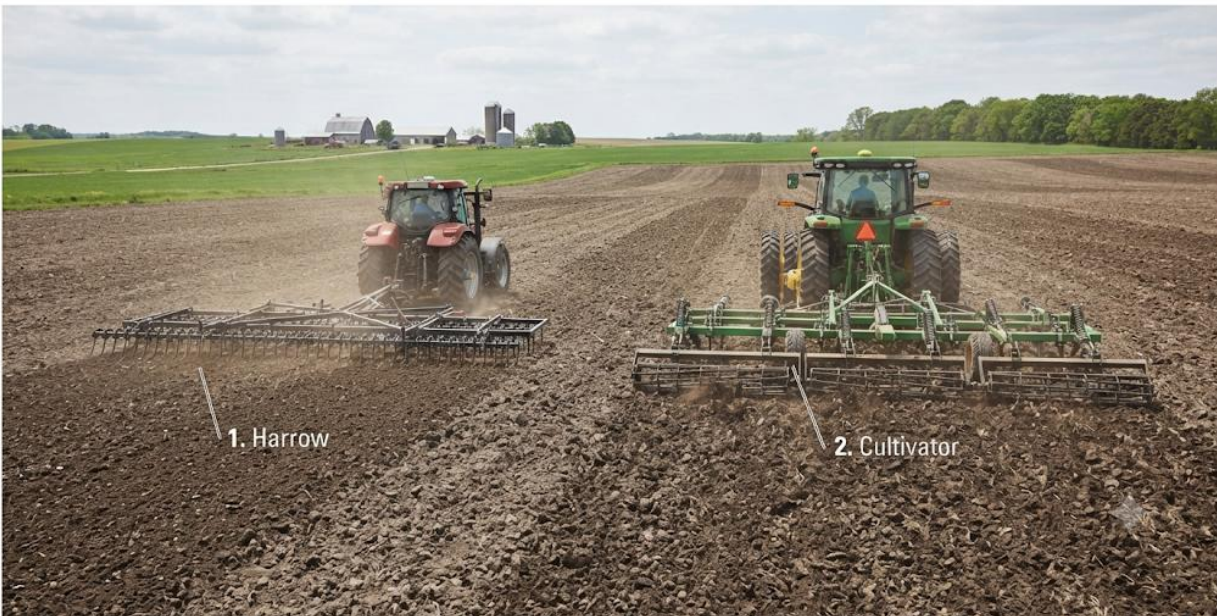
Plate 2.1 Secondary tillage implements in operation
