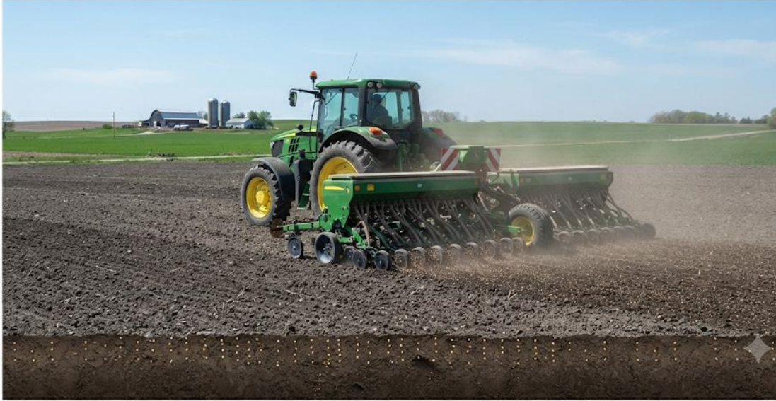
Plate 5.2 Mechanized planting with seed drill
