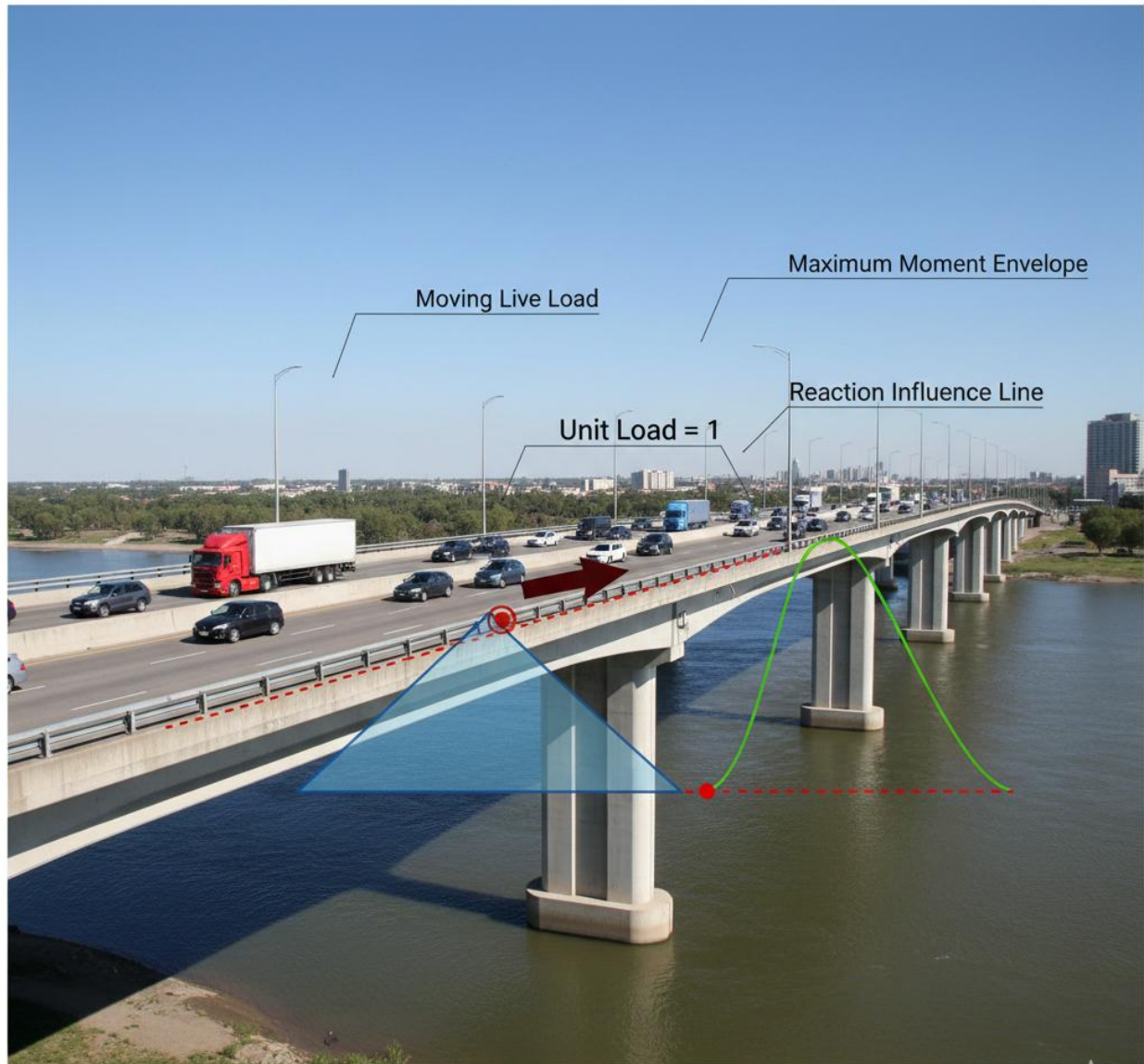
Plate 4.1 Practical application of influence lines in bridge design
