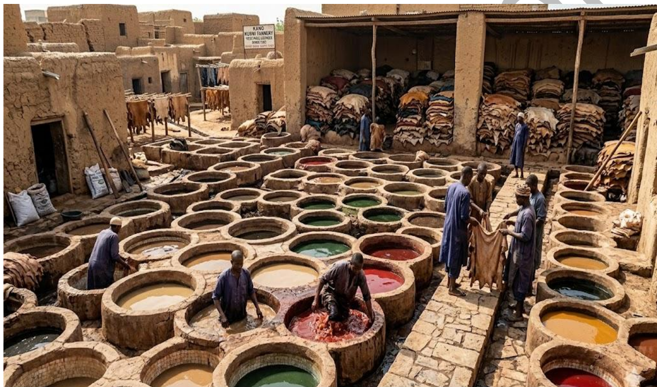
Figure 2.3: Photograph of the traditional Kano tannery showing vegetable tanning pits and workers processing hides
