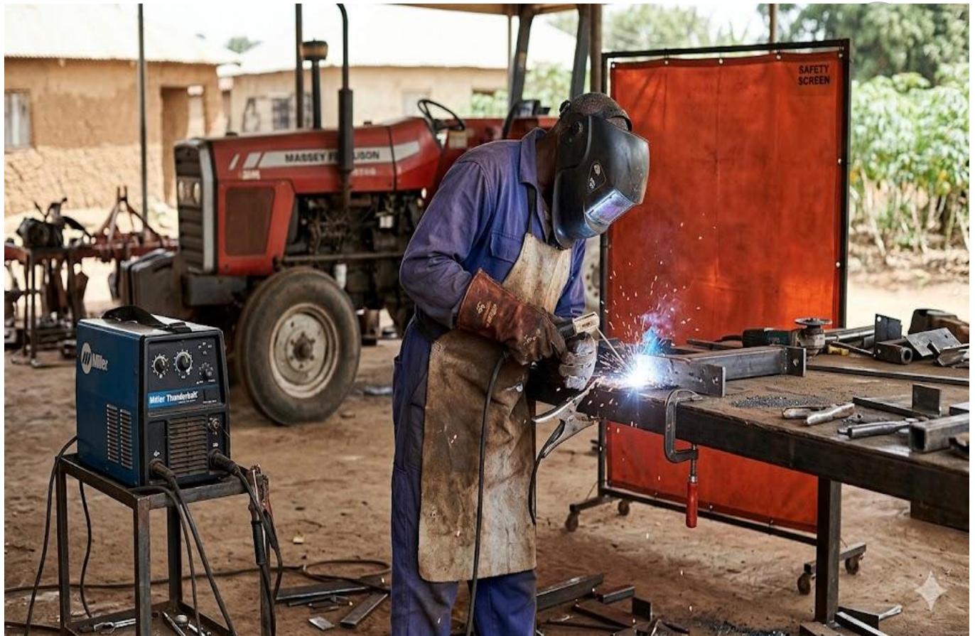
Plate 2.1: Shielded metal arc welding (stick welding) in an agricultural workshop
