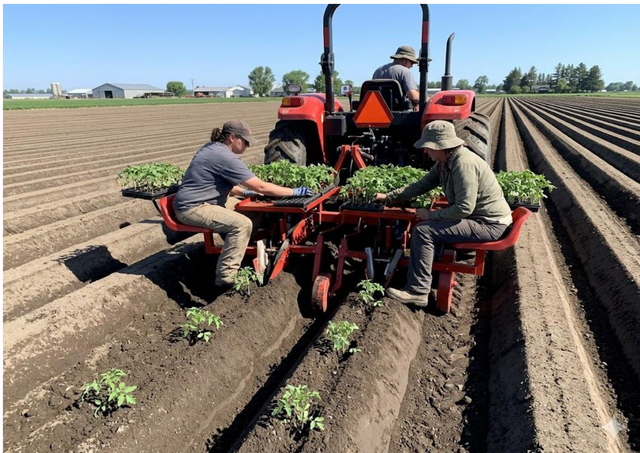
Plate 3.2: A two-row semi-automatic transplanting machine in operation transplanting tomato seedlings into prepared ridges
