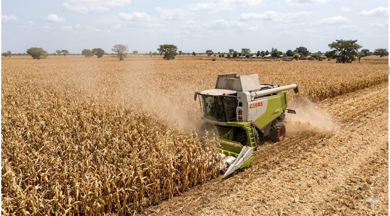
Plate 4.1: A self-propelled combine harvester harvesting maize in a Nigerian savanna commercial farm
