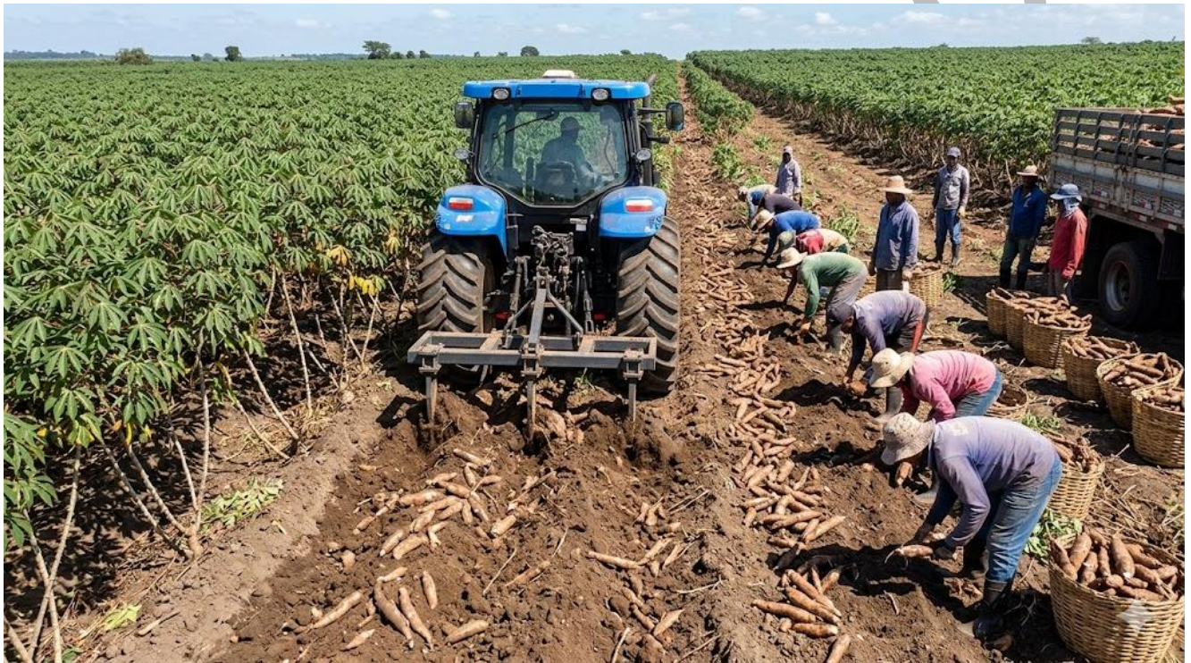
Plate 4.3: A tractor-mounted cassava harvester with a subsoil lifting bar loosening roots for manual collection
