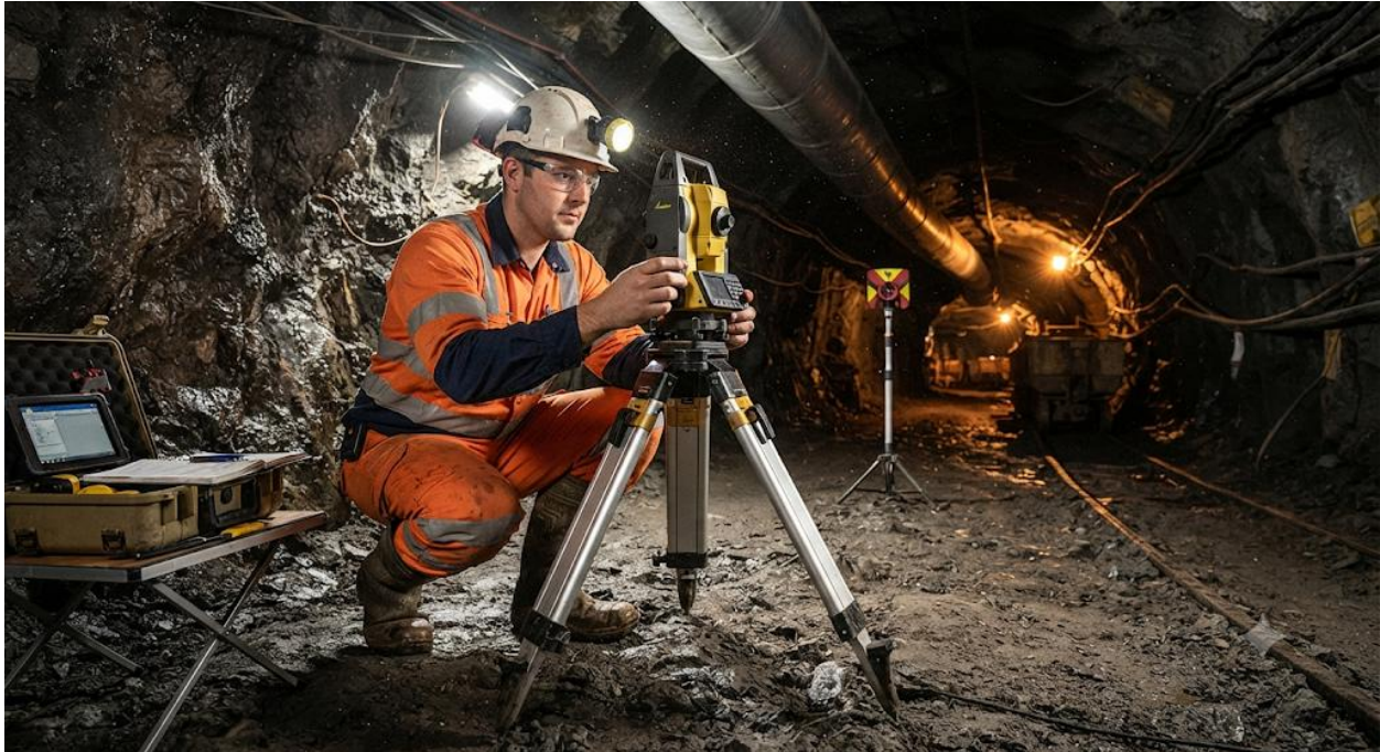
Photograph of a surveyor setting up a theodolite in a mine. Plate 1.2: Surveyor operating a mining theodolite
