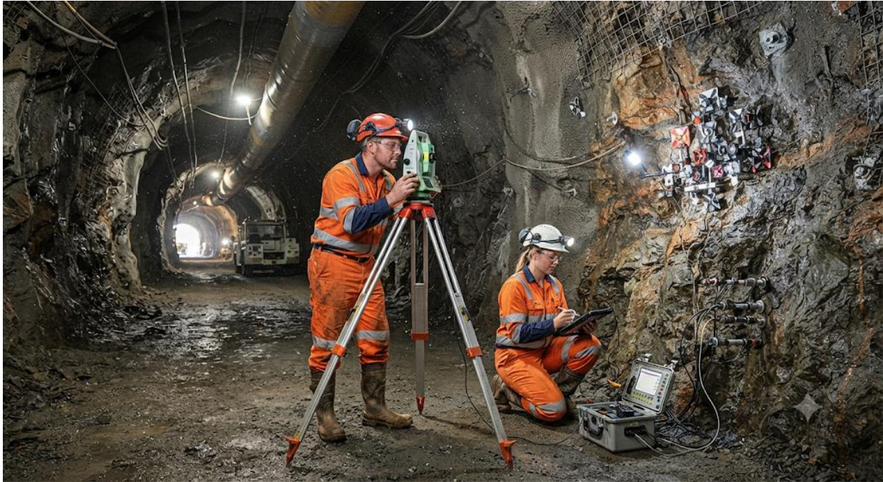
Photograph of surveyors monitoring rock displacement underground. Plate 3.3: Monitoring rock displacement in underground mines
