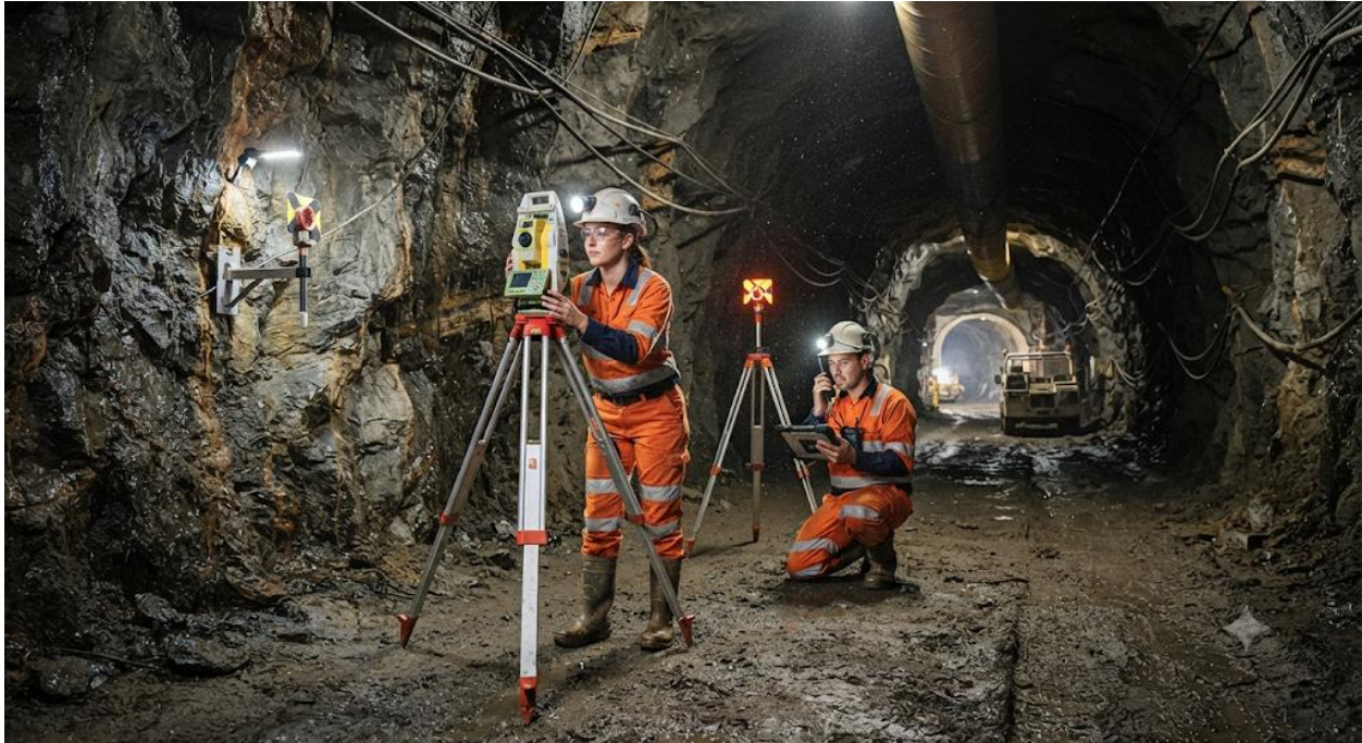
Photograph of surveyors working in an underground tunnel. Plate 3.1: Tunnel surveying in underground mines
