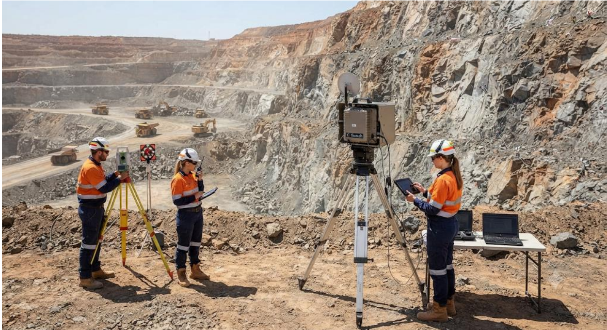
Photograph of slope monitoring equipment in a quarry. Plate 2.3: Monitoring slope stability in quarry operations
