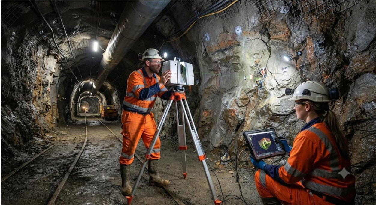
Photograph of surveyors using laser scanning equipment underground. Plate 4.3: Surveying techniques for monitoring deformation
