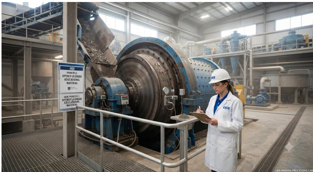
Photograph of a ball mill in operation Plate 2.2: Ball mill used in mineral processing
