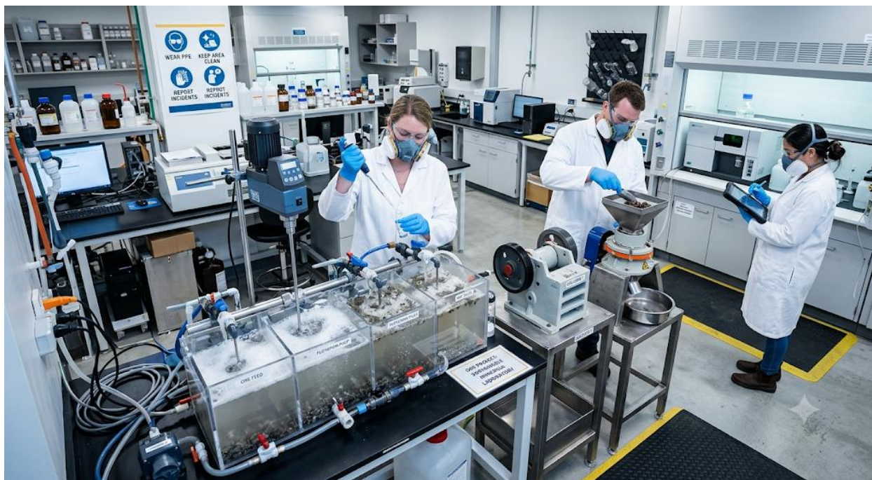
Photograph of mineral processing laboratory with flotation cells, crushers, and PPE in use Plate 5.3: Laboratory equipment and safety protocols
