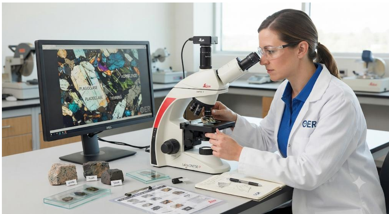
Photograph of a petrographic microscope in use Plate 1.3: Petrographic microscope for mineralogical analysis
