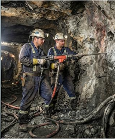
PORTABLE DRILL: Handheld Pneumatic Drill, used for exploration and small-scale blasting in underground mining. Compact, flexible, operated manually.
