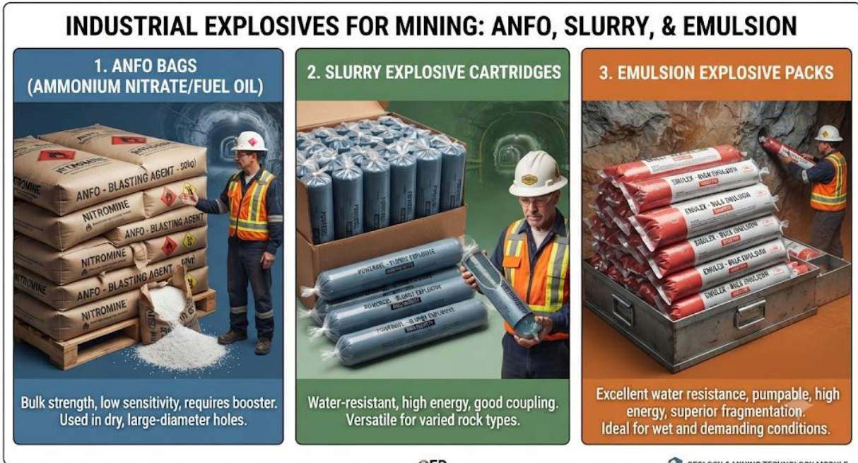
Image showing industrial explosives used in mining (ANFO bags, slurry cartridges, emulsion packs) Caption: Plate 3.1 Industrial explosives used in mining and construction
