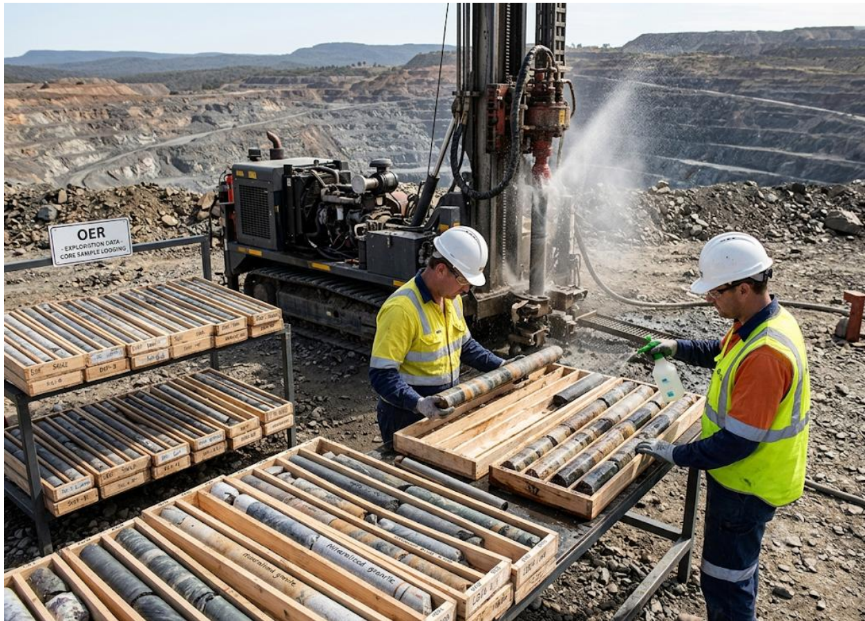
Image showing diamond drilling equipment and recovered core samples Caption: Plate 1.2 Diamond drilling rig and core samples
