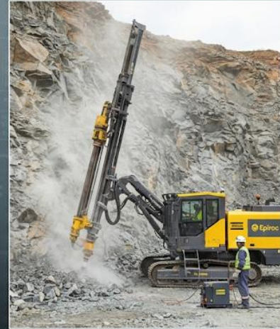
PERCUSSIVE DRILL: Track-mounted drill, uses rapid hammer impacts combined with rotation to fracture rock. Efficient for hard rock drilling.
