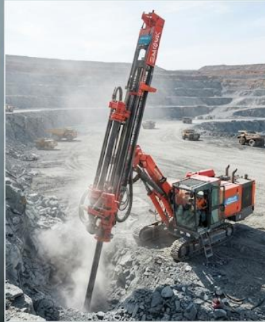
ROTARY DRILL: Large track-mounted rig, uses continuous rotation and down pressure to crush rock. Ideal for large diameter holes in open-pit mining.
