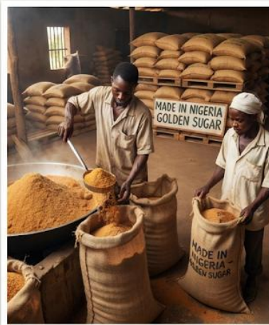
STAGE 3: CRYSTALLIZATION AND PACKAGING - The concentrated syrup cools and crystallizes into raw brown sugar, which is then packed for distribution.
