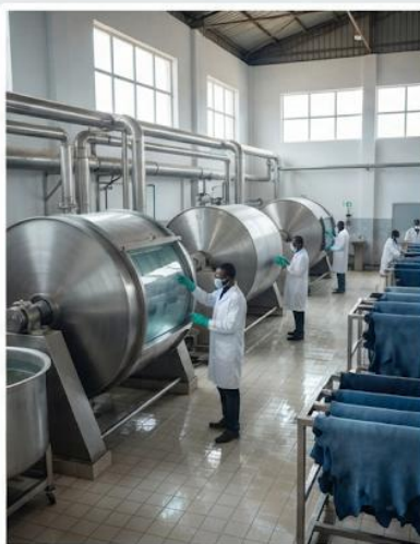
MODERN LEATHER TANNING FACTORY: Nigerian technicians in a clean facility managing chemical processing of hides in large stainless steel drums in Kano.
