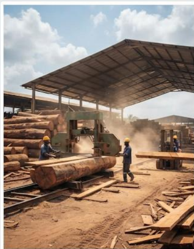
SAWMILL TIMBER PROCESSING: Nigerian workers operating an industrial bandsaw to cut large hardwood logs into planks in a facility in Ogun State.
