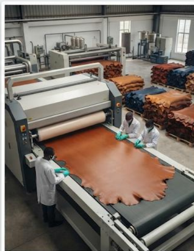
LEATHER FINISHING: Nigerian operators inspecting dyed and finished leather as it passes through an automated application machine in Kano.
