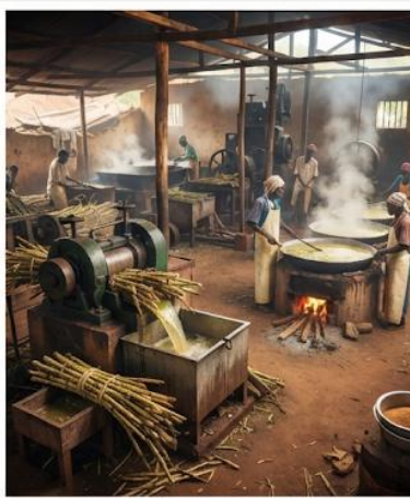
STAGE 2: MILLING AND BOILING - Cane juice is extracted and boiled in open pans to evaporate water and create concentrated syrup.
