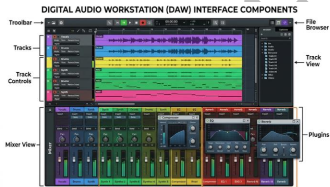
Figure 2.2 Basic layout of a Digital Audio Workstation
