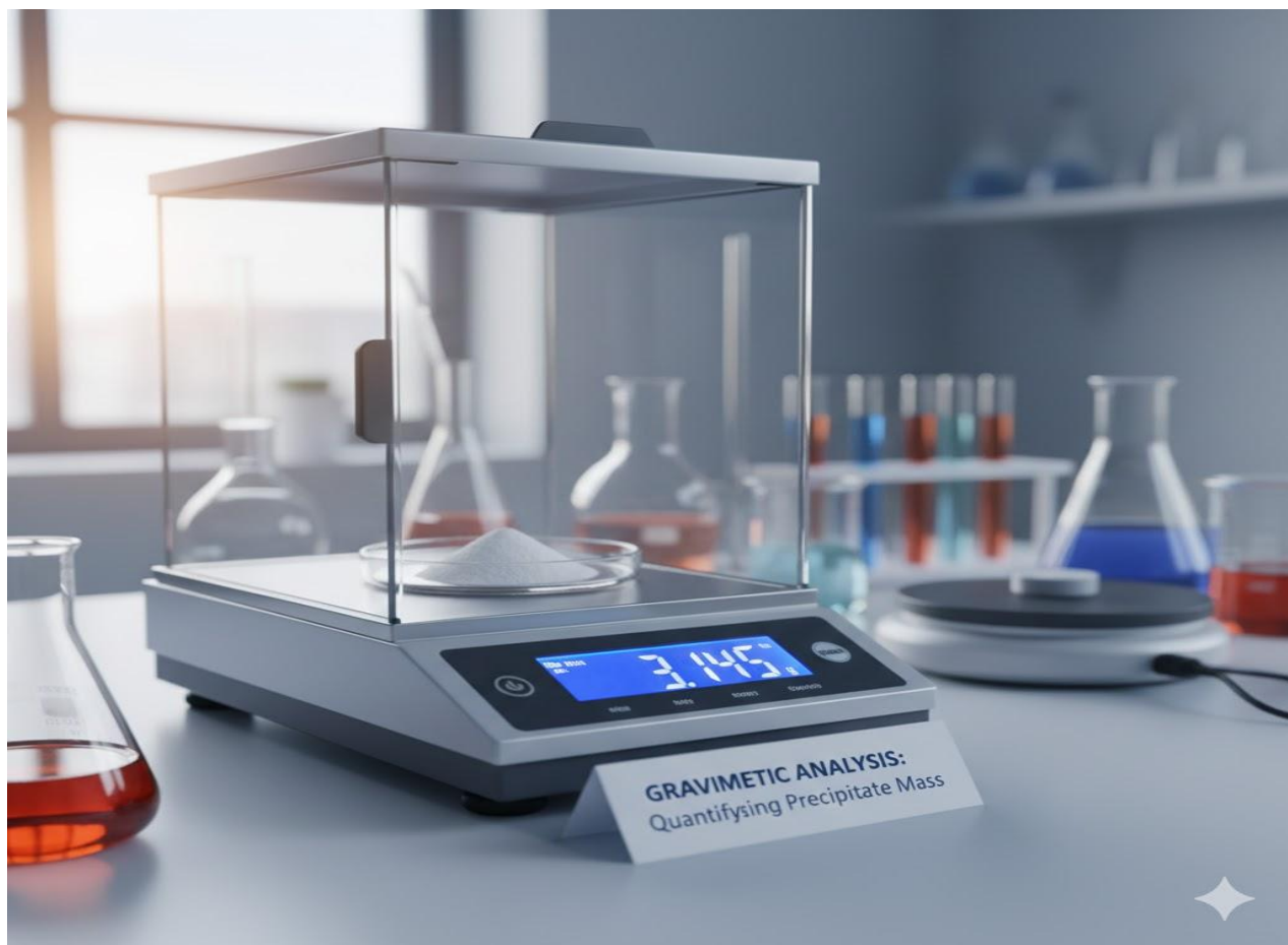
Figure 4.1: Analytical balance weighing a precipitate to illustrate the principle of gravimetric analysis.
