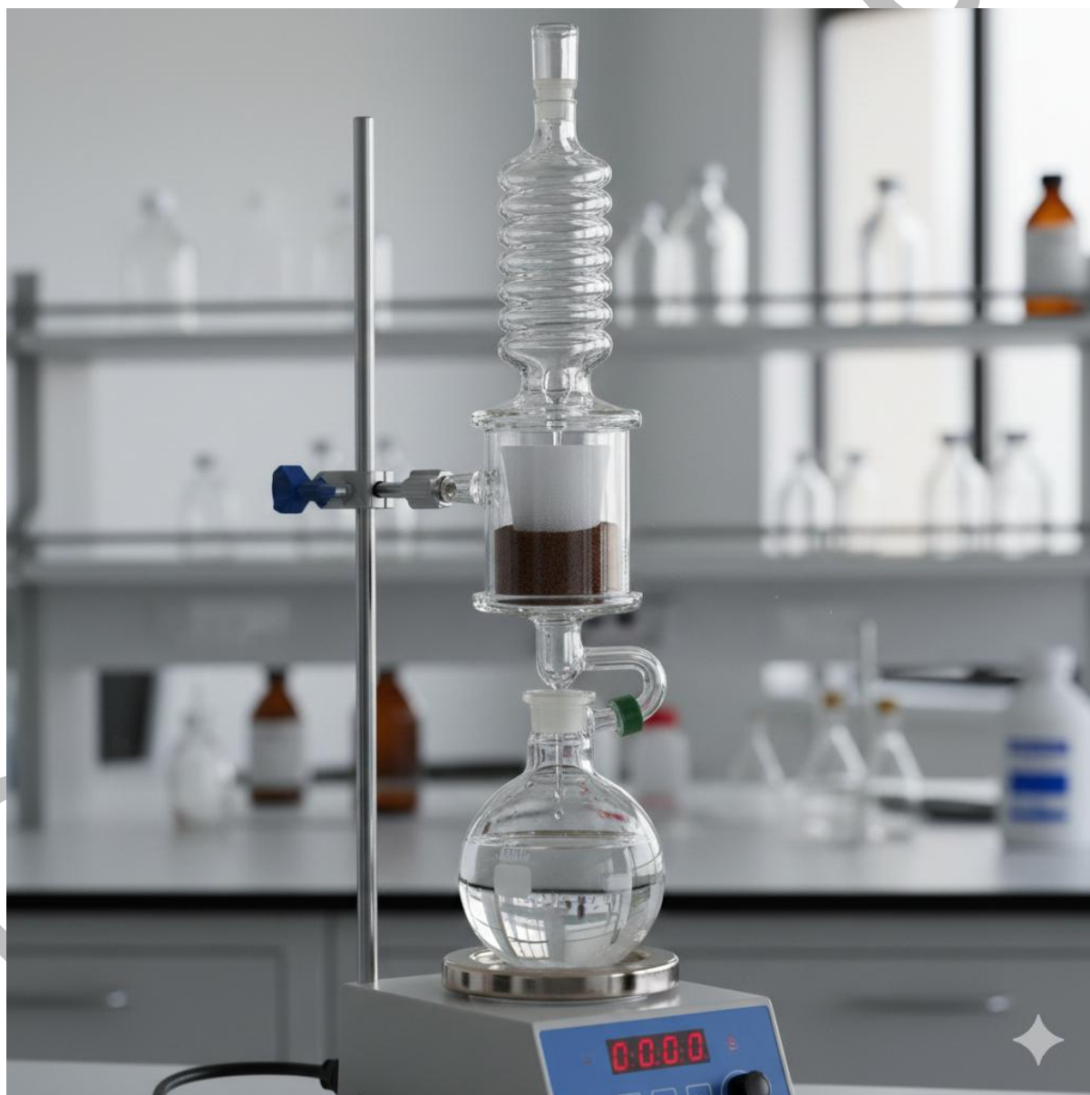
Plate 1.2 Soxhlet apparatus for crude fat determination
