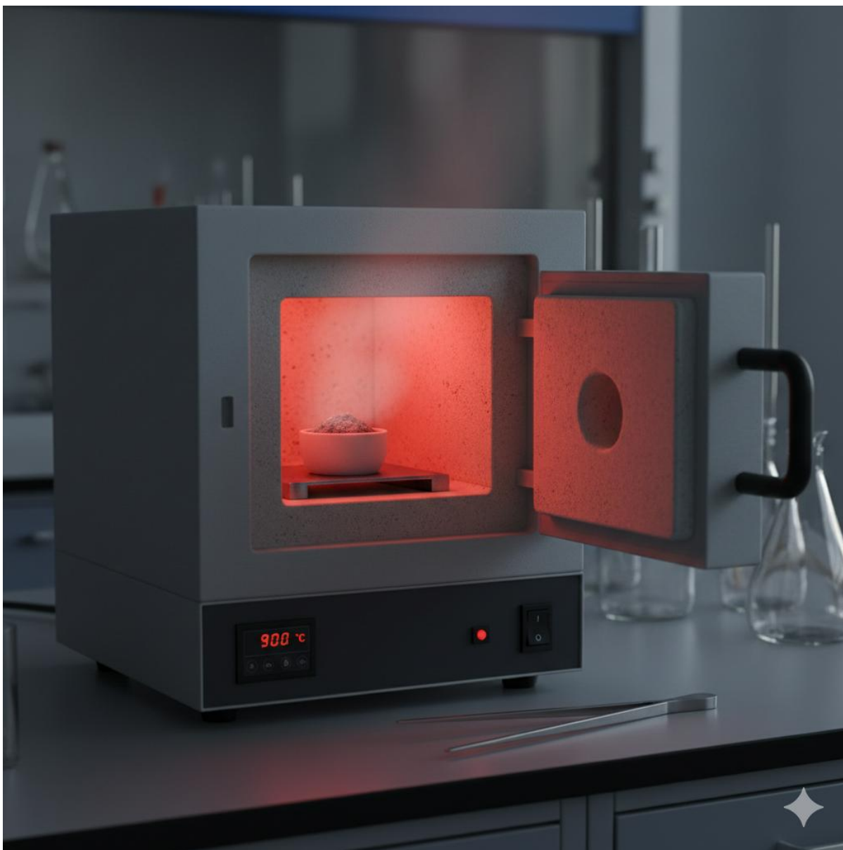
Plate 1.1 Muffle furnace for dry ashing of food samples
