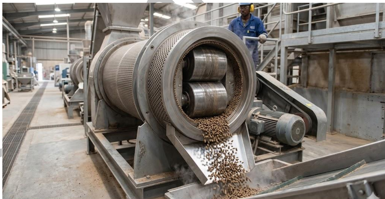
Plate 5.1: Ring-die pellet mill in a commercial fish feed factory showing the die and roller assembly Plate 5.1: Ring-die pellet mill in a commercial fish feed factory showing the die and roller assembly
