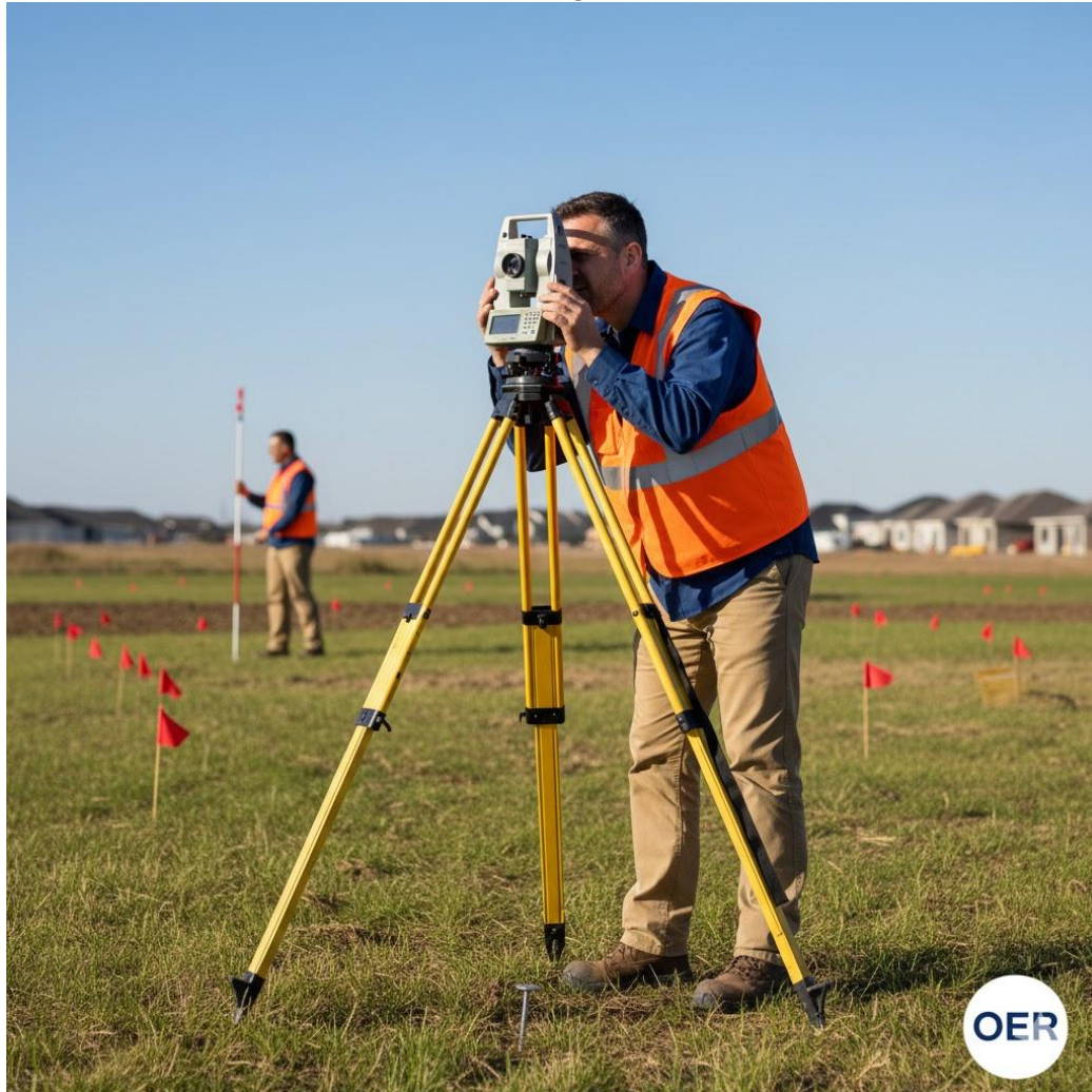
Plate 3.2: Conducting a theodolite traverse:
