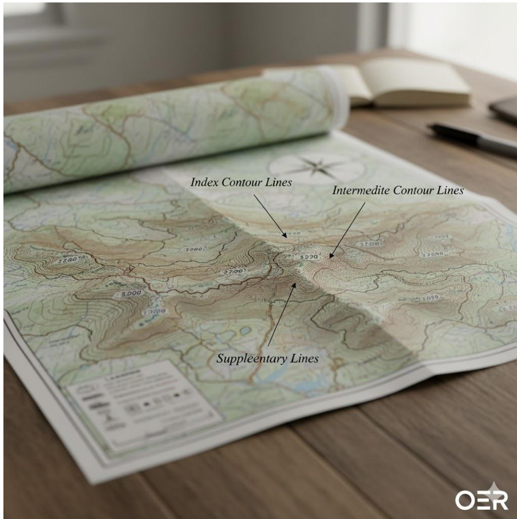
Plate 2.1: Types of contour lines on a topographic map:
