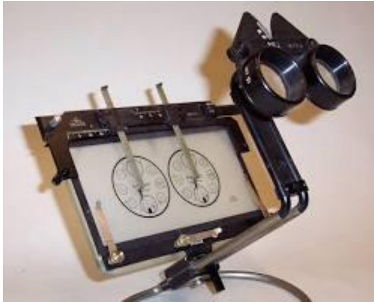
Plate 5.3: Stereoscope for stereoscopic vision
