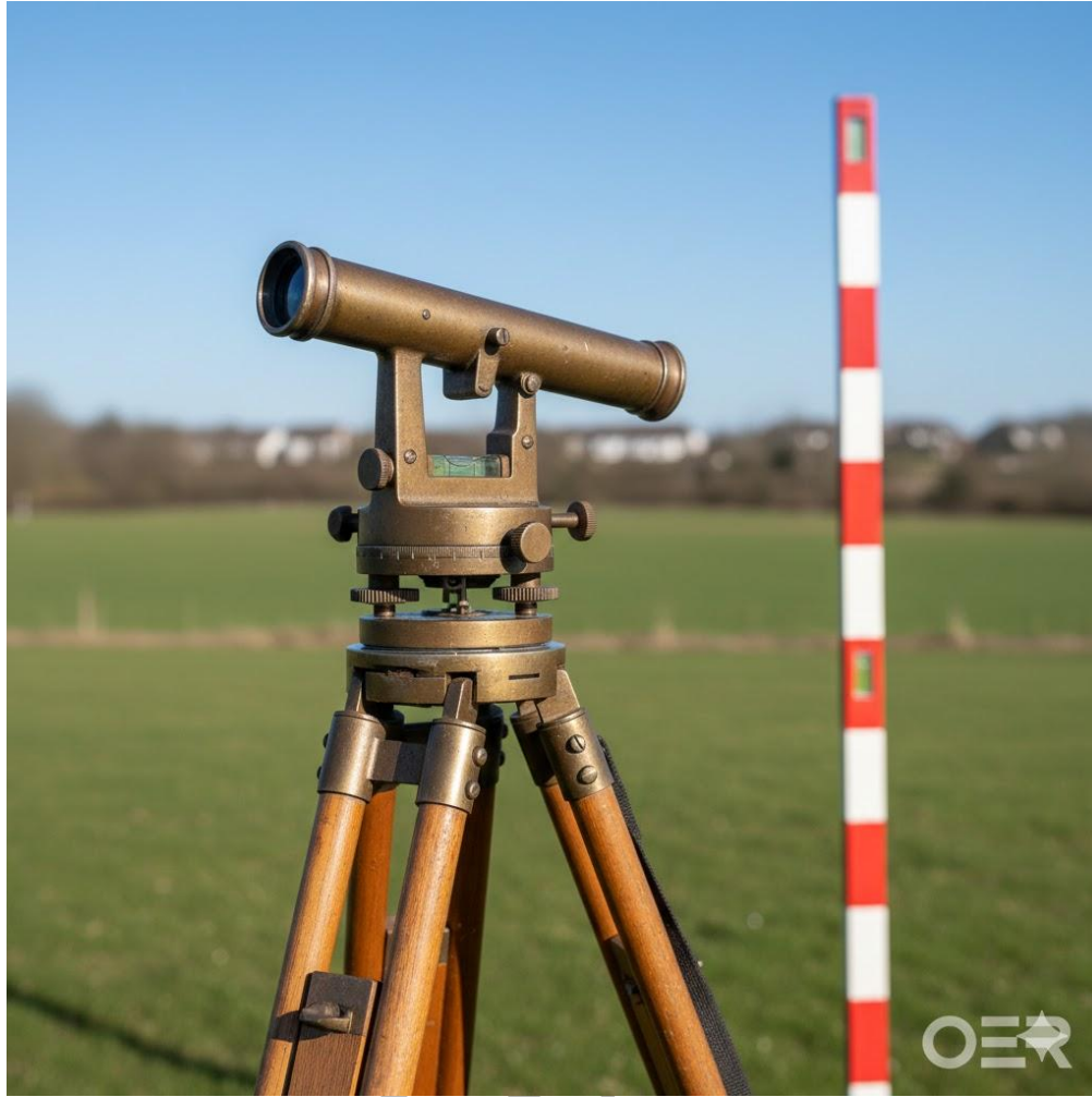
Plate 4.1: Dumpy level and staff used in levelling:
