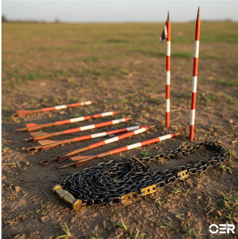
Plate 1.1: Common instruments used in chain surveying:
