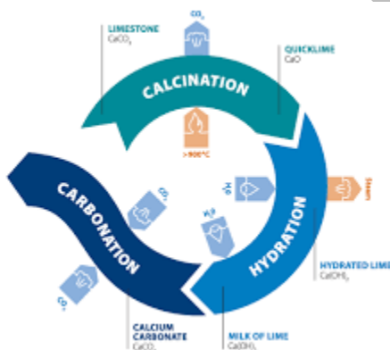
Figure 5.4: Types of lime and their production process
