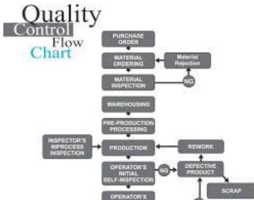
Figure 2.5: Stages of quality control in steel production
