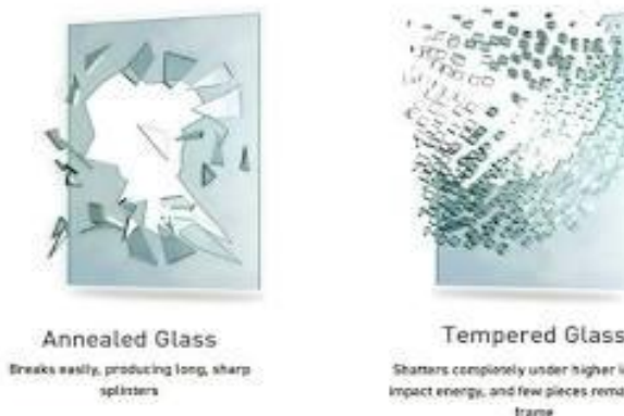
Figure 5.3: Types of glass in construction
