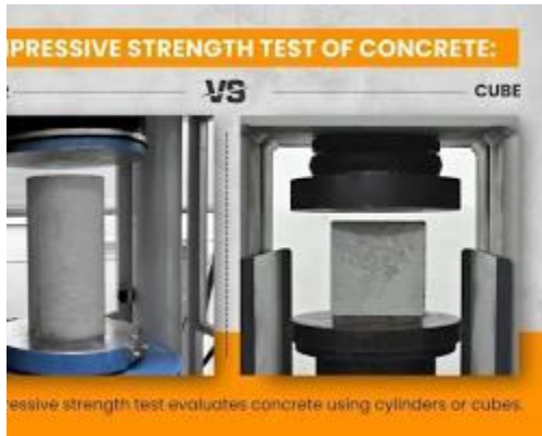
Plate 1.4: Testing compressive strength of concrete cubes
