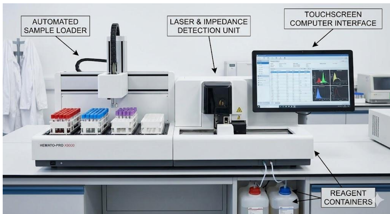
Plate 4.1: Automated haematology analyser and its components
