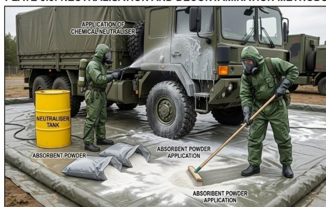
METHODS FOR DECONTAMINATING EQUIPMENT USING CHEMICAL NEUTRALISERS AND ABSORBENT POWDERS
