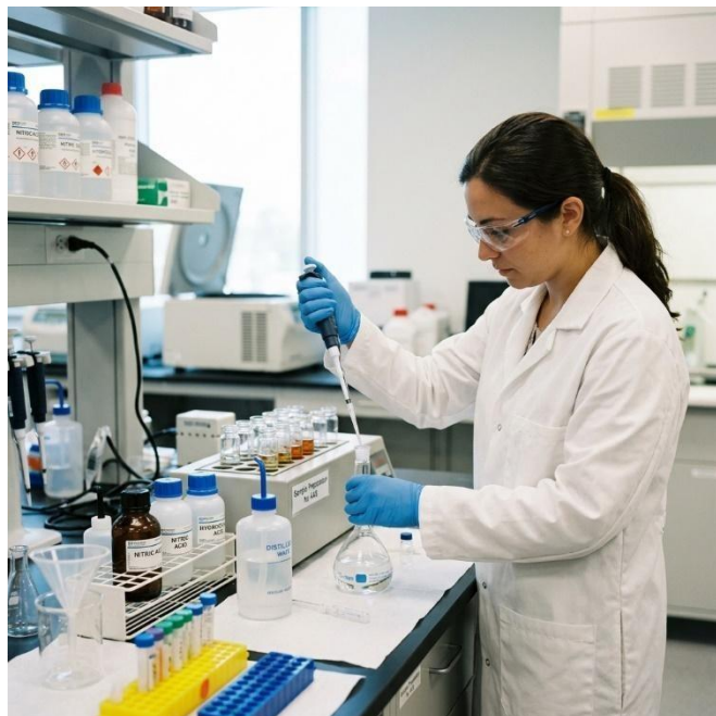
Image showing laboratory technician preparing samples for atomic absorption analysis. Plate 2.3: Sample preparation for atomic absorption spectrometry
