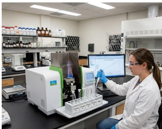
Plate 5.2: Use of standard solutions in atomic absorption spectrometry.
