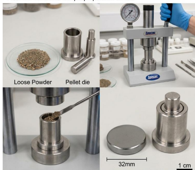
Plate 4.2. Powdered sample preparation for XRF
