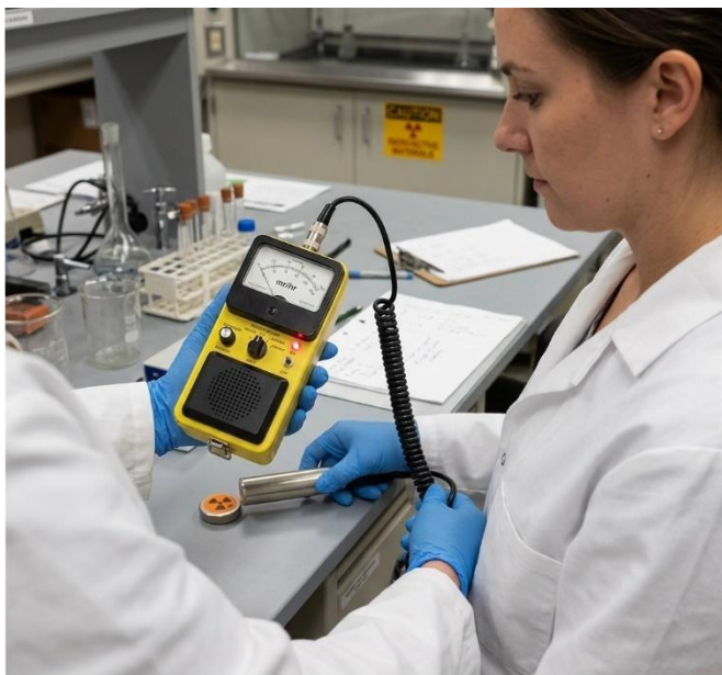
Plate 4.3 Geiger–Müller counter for radiation detection. Image showing a Geiger–Müller counter being used to measure radiation. Plate 4.3 Geiger–Müller counter for radiation detection. “Geiger–Müller counter radiation detection OER”
