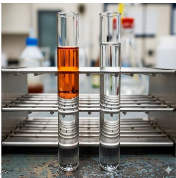
Plate 5.1: Bromine water test for alkenes
