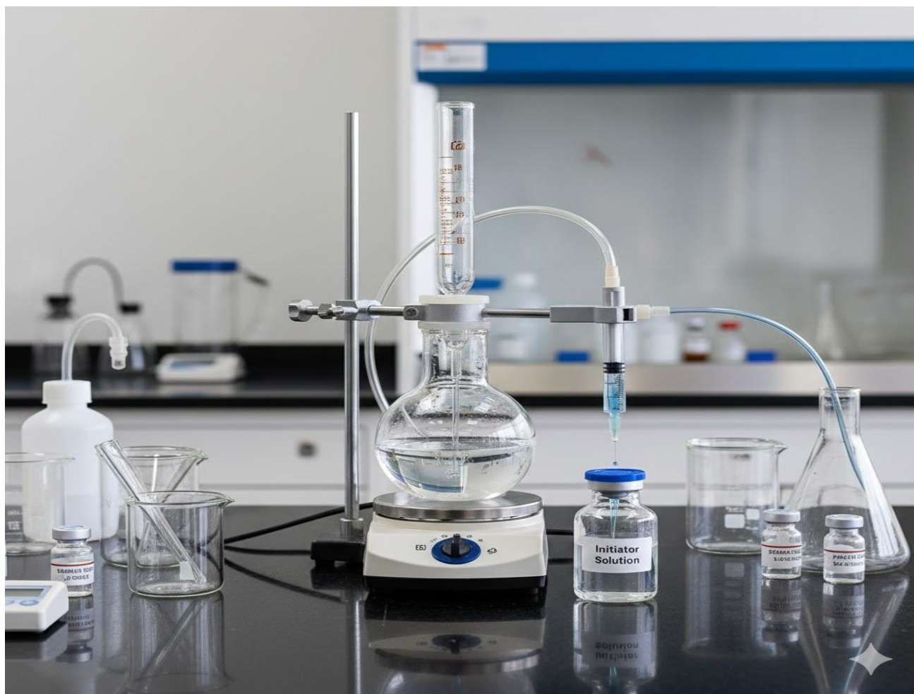
Plate 1.1 Laboratory setup for free radical polymerisation
