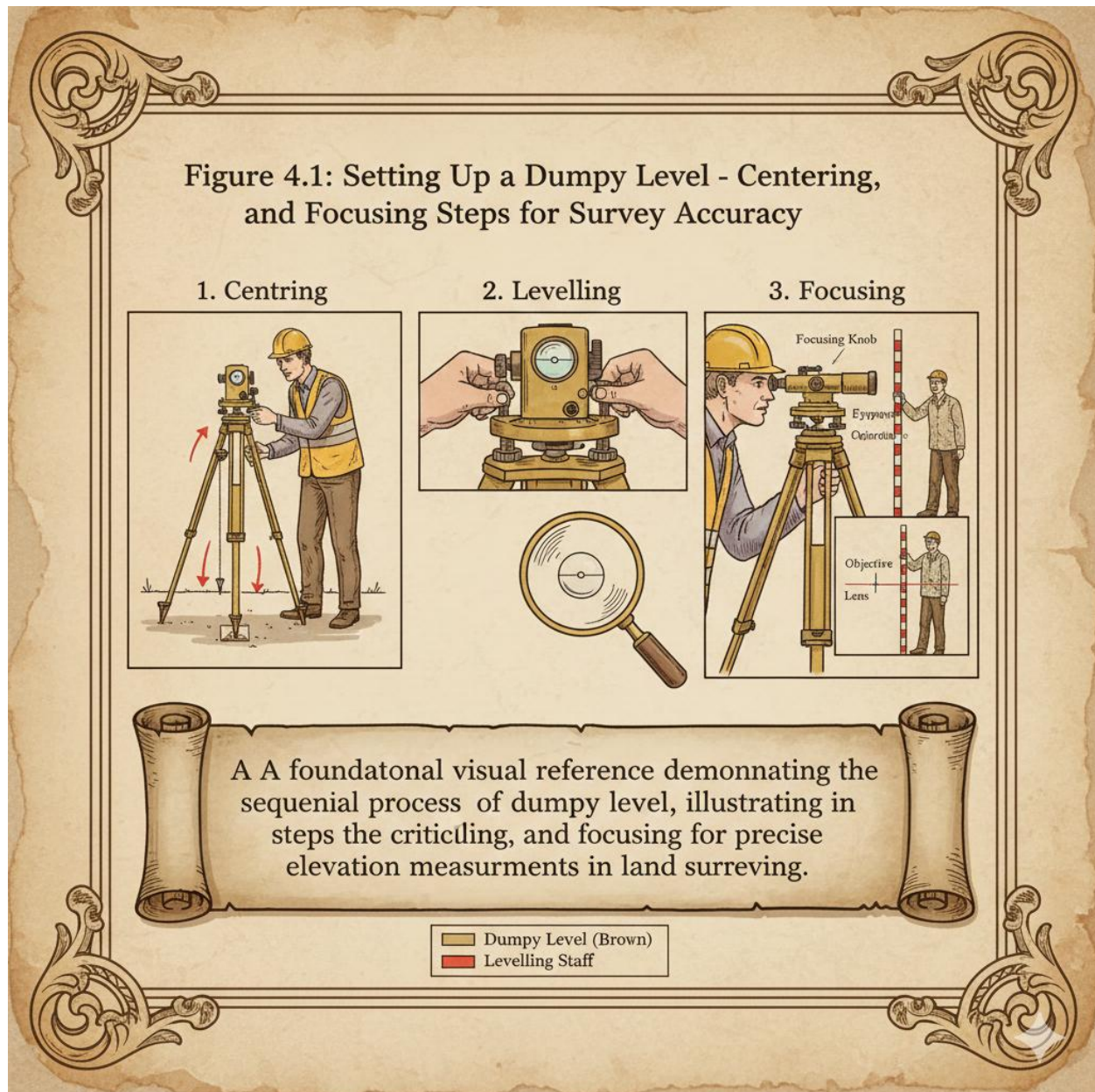
Diagram showing the setup of a dumpy level with centring, levelling, and focusing steps. Figure 4.1: Setting up a dumpy level
