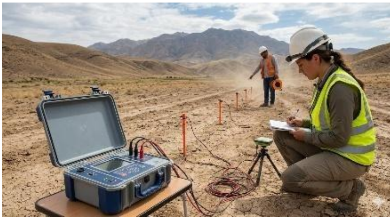
Plate 3.2: Resistivity meter and electrode setup
