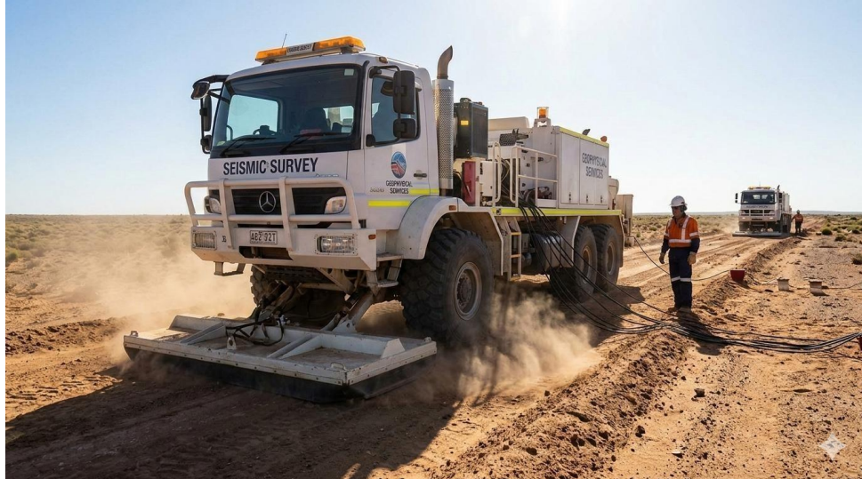
Plate 2.1: Seismic vibrator truck generating controlled
