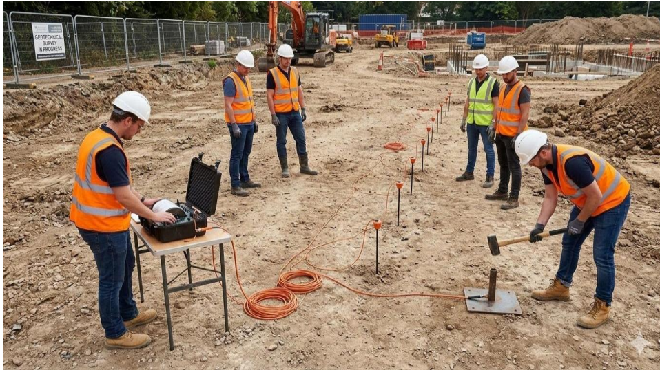
Plate 2.4: Shallow seismic survey for engineering purposes
