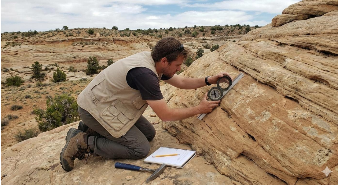
Plate 5.2 Field data collection using a compass-clinometer.
