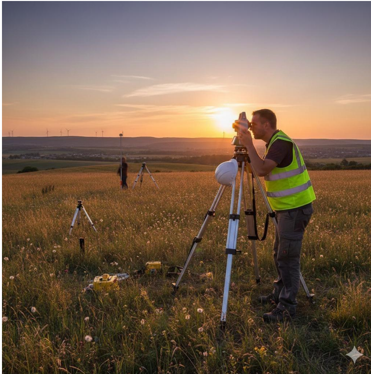
Plate 1.4 Surveyor using an EDM device for precise measurement.
