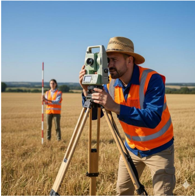
Plate 1.3 Surveyor using a theodolite to measure angles.
